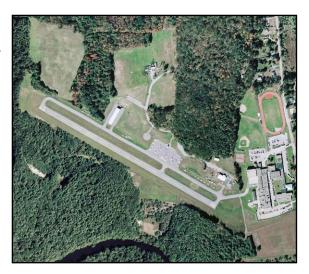
The airfield facilities at Danielson Airport include a 2,700-foot long paved runway (Runway 13-31), full-parallel taxiway, and associated lighting and visual aids (e.g., wind sock). An Automated Weather Observing System (AWOS) was recently installed that provides surface weather conditions to pilots via a radio frequency.
